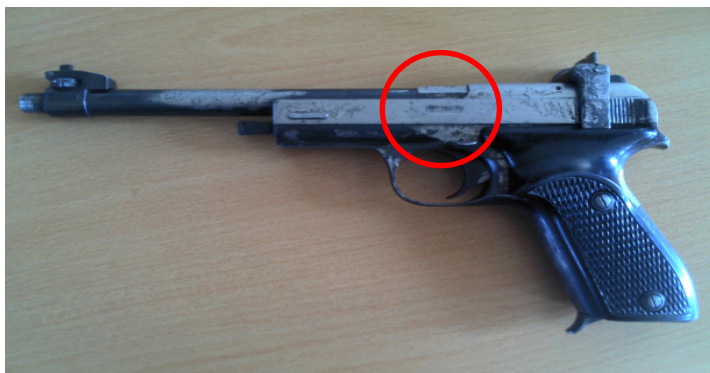
(a) Photo of the object — the MCM pistol with the removed serial number
