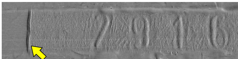
(b) Additional magnetization of the object placed on the pivoted arms of the magnetizing staple (according to the scheme given in Figure 3)
