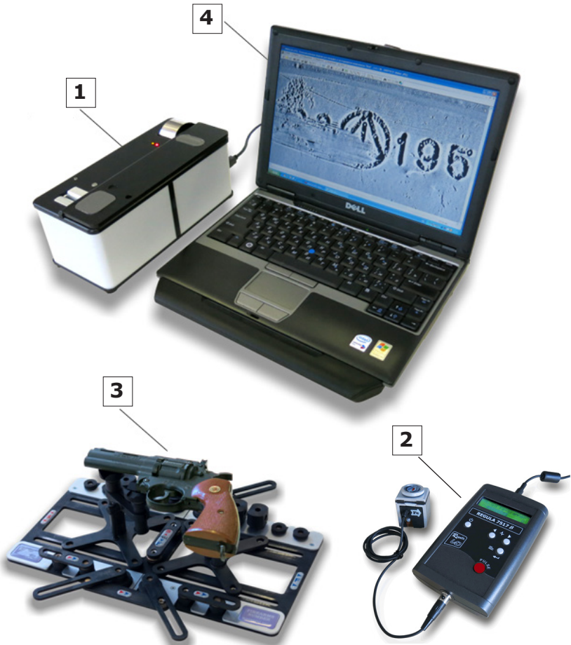
Figure 1. HSS general view: 1 – magneto-optical device Regula 7517A; 2 – eddy-current magnetographing device Regula 7517B; 3 – magnetizing equipment Regula 7517C; 4 – PC (laptop).
