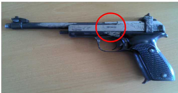
(a) Object photo — the MCM pistol with the removed number
