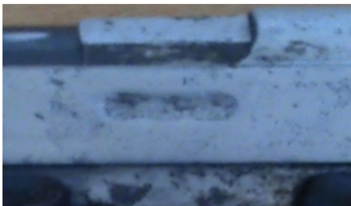
(b) Photo of the number platform — elements of the number are not recognized
