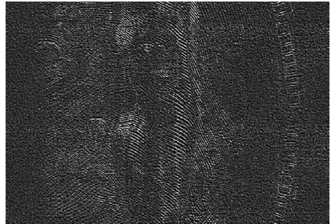
Magnetic-optical visualization of the same fragment. This is result of image software processing: negative presentation and 3D processing make magnetic stroke more obvious.
