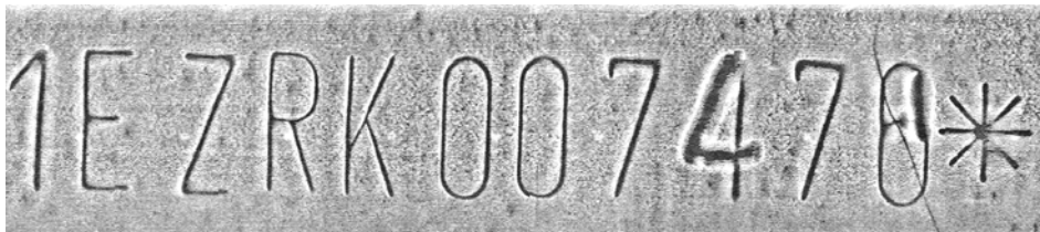
Fig.5. MOV of a fragment of an automobile body number platform with fragments of primary numbers (... 1EZRK007176), changed by a method of filling the crosspieces by fusible metal (paint cover was not removed).
