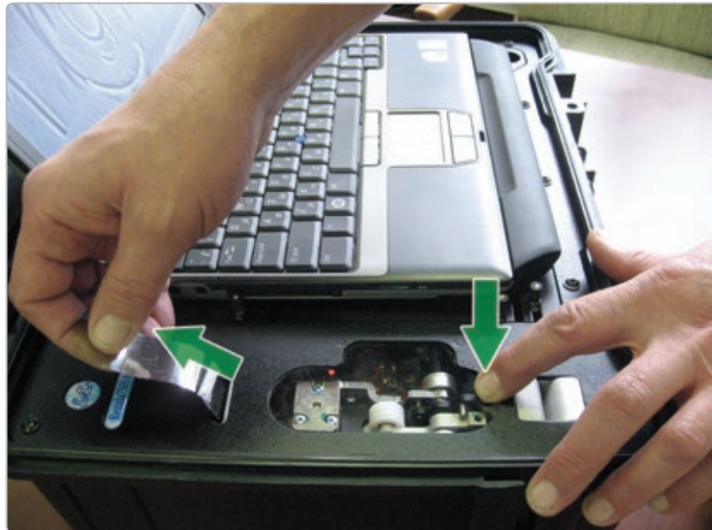
Manual extraction of the magnetic tape from OMB tape drive
